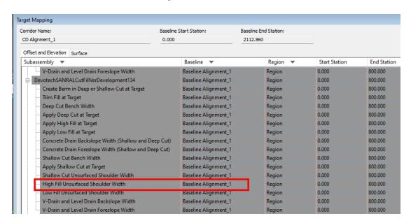
2. Fixed the bug that caused the unsurfaced shoulder in high fill condition to not to change the shoulder width if the high fill drain was not used.
