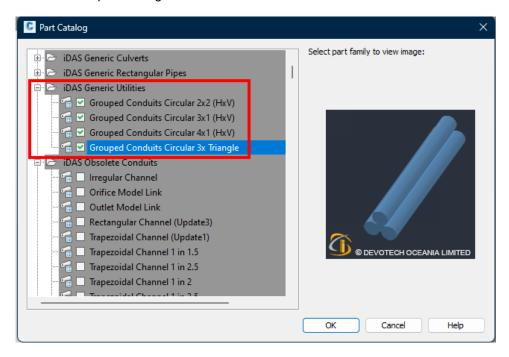
These conduits can be used for various services and since they are modeled in Part Builder, they can also be used for the clash detection.
