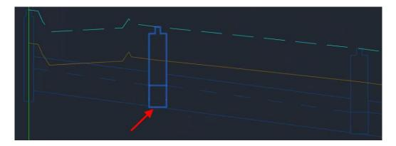
This visual appearance can be achieved by setting the structure's floor thickness to 0 mm. Hower, some structure families did not offer 0 mm thickness to be used for floor thickness:
