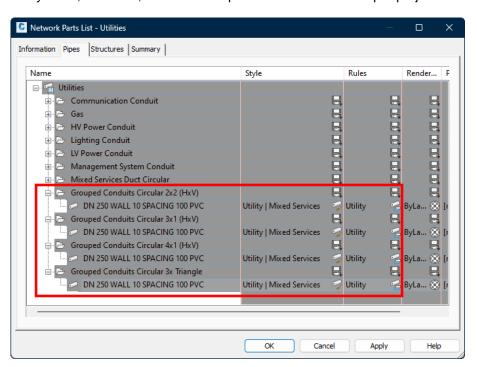
When importing different sizes, the spacing between pipes can be defined for each size:
