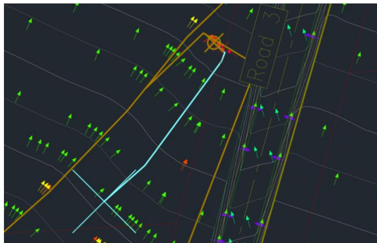
Figure 5: Flow Path Created using Water Drop Function in Autodesk Civil 3D
